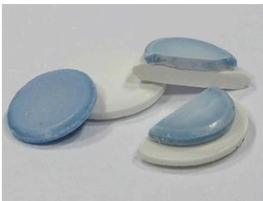
**Figure 1.** Final PBs, blue the enamel-like and white the dentin-like PBs. On the right side assembled specimens are displayed.
