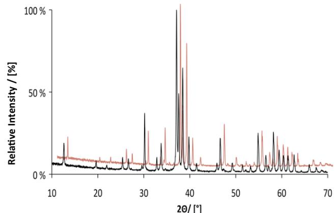
**Figure 5.** XRD diffractogram of the enamel-like PB (black), crystallinity grade comparable with pure crystalline hydroxyapatite (red).
