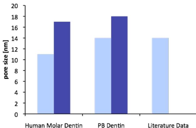
**Figure 4.** Measured pore size by (•) MIP and (◦) BET of human coronal molar dentin, PB dentin and literature data [2].
