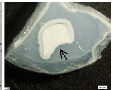
**Figure 3.** Enamel-like PB with an artificial lesion (arrow).
